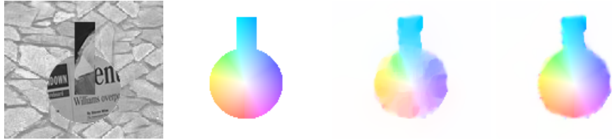
Fig. 2. Results for a pure rotation movement (3 degree anti-clockwise). From left to right: (a) First frame. (b) Optical flow ground truth. (c) Estimated optical flow using the TV regularizer. (d) Estimated optical flow using the proposed regularizer.
